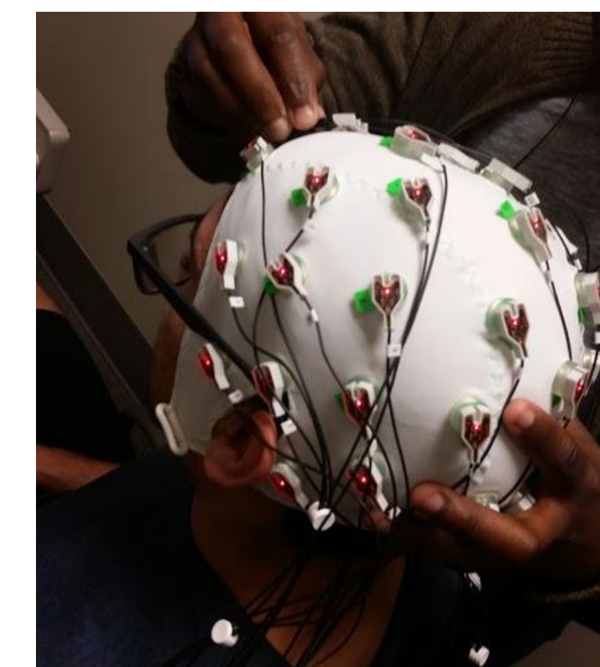
Figure 3. 32 electrode EEG cap used in ELDEN lab.
